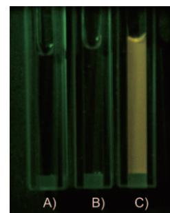
Figure 3. A photograph of A) D1/N , B) H2AD/H2B and C) H6AD/H6B at RT. Solution conditions were as follows: [DNA] = 1.0 \mu\text{M} , [NaCl] = 100 mM, pH 7.0 (10 mM phosphate buffer). Excitation wavelength: 520 nm.
